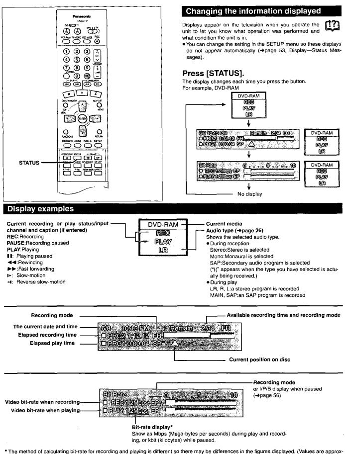
\* The method of calculating bit-rate for recording and playing is different so there may be differences in the figures displayed. (Values are approximate.)
